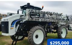
**2014 GVM E370 Prowler,** 393 demo hours, Cummins QSL9 370 hp diesel engine, 1800 gal. SS tank, 4 chemical induction tanks, 60/90 ft booms, dual, low, and high volume boom lines for suspension fertilizer, high volume Ace pump, Viper Pro, Phoenix 200 receiver, SmarTrax 3D, UltraGlide, 380/90R46 tires. Includes 5-year warranty, began May 15, 2017.
