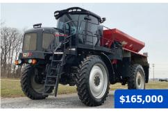
**2017 RBR Vector 300**, 2958 hours, Cummins QSB 8.3 300 hp diesel engine, Allison 6-speed auto. trans., New Leader L4000G4 spreader body, Viper Pro, A/C, air ride seat, 380/90R46 tires (50% remains). Also includes (4)Firestone 650/65R38 floater tires. SN: M1700598 (PA) **No. U1422**
