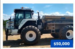
**2010 GVM 9275 Prowler,** 5099 hours, Cummins QSB6.7L 275 hp diesel engine, auto. Funk 10-speed powershift trans., 9.5 ton GVM Double Duty spreader body, Raven Viper 4, A/C, AM/FM radio, air ride seat, manual roll tarp, includes 650/75R32 front (10% remains) and 800/65R32 rear (60% remains) Goodyear floater tires. **Frame sandblasted and painted, Winter 2019.**
