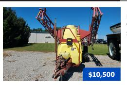
**2005 Hardi Navigator 1100,** 540 PTO pump, 1100 gal., 80 ft booms with plastic boom lines, single nozzle body, 20 in. nozzle spacing, 4-section shutoff valve, foam marker, chemical inductor, manual adjustable axles, 12.2-42 Titan tires (35% remains).
