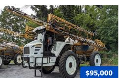
**2011 GVM 9275 Prowler,** 3994 hours, Cummins QSB6.7L 275 hp diesel engine, Funk 10-speed powershift trans., 1450 gal. SS tank, 70/90 ft booms with SS boom lines, 15 in. nozzle spacing, 5-section shutoff valve, triple body nozzles, Raven Viper Pro, parallel swatching, AutoSteer, A/C, AM/FM radio, air ride seat, 380/90R46 Trelleborg tires (30% remains), includes set of floater tires not pictured.
